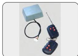
Remoter: two button transmitter, inner antenna, distance>30m
